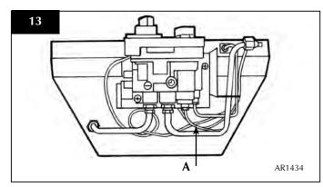
• Undo the thermocouple nut in the pilot unit by half a turn. This will release the thermocouple.
